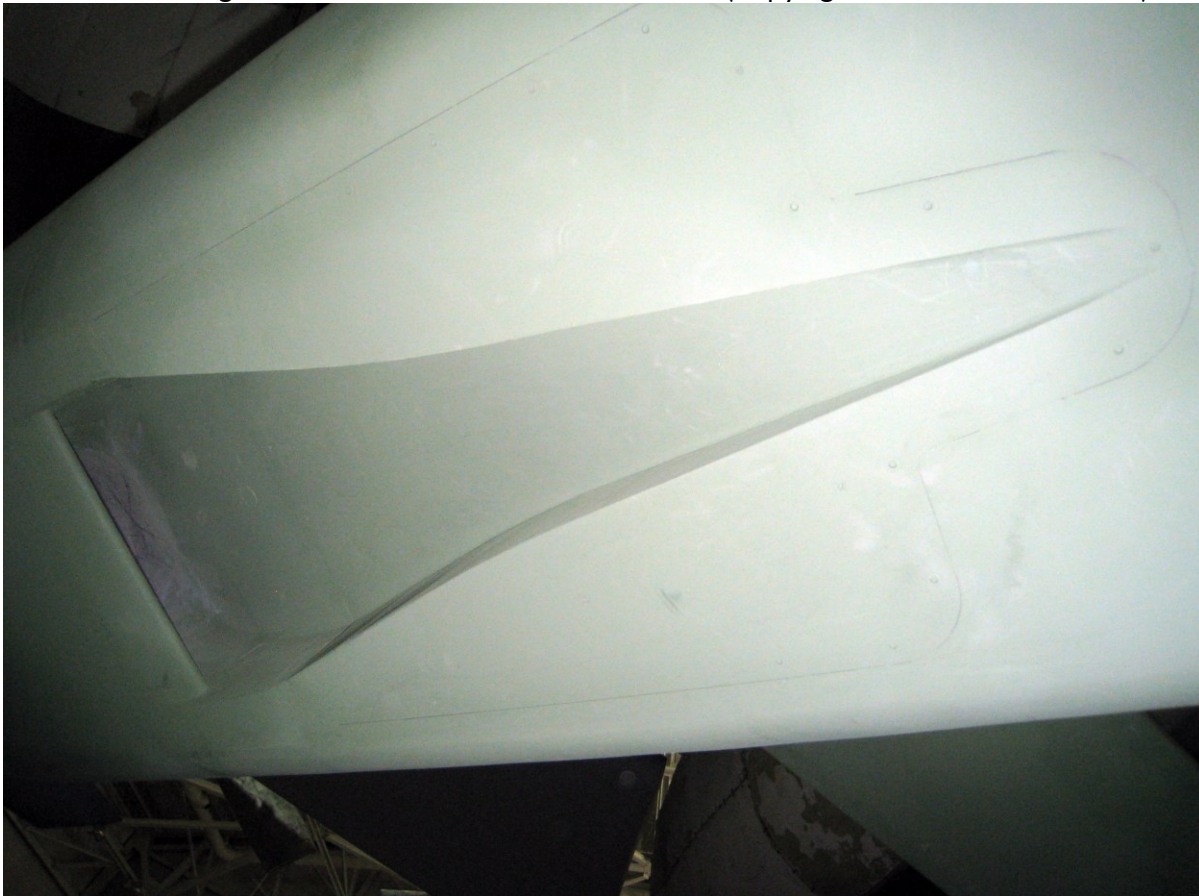
The flush NACA inlet on the underside. (copyright 2012 Scott Lowther)
