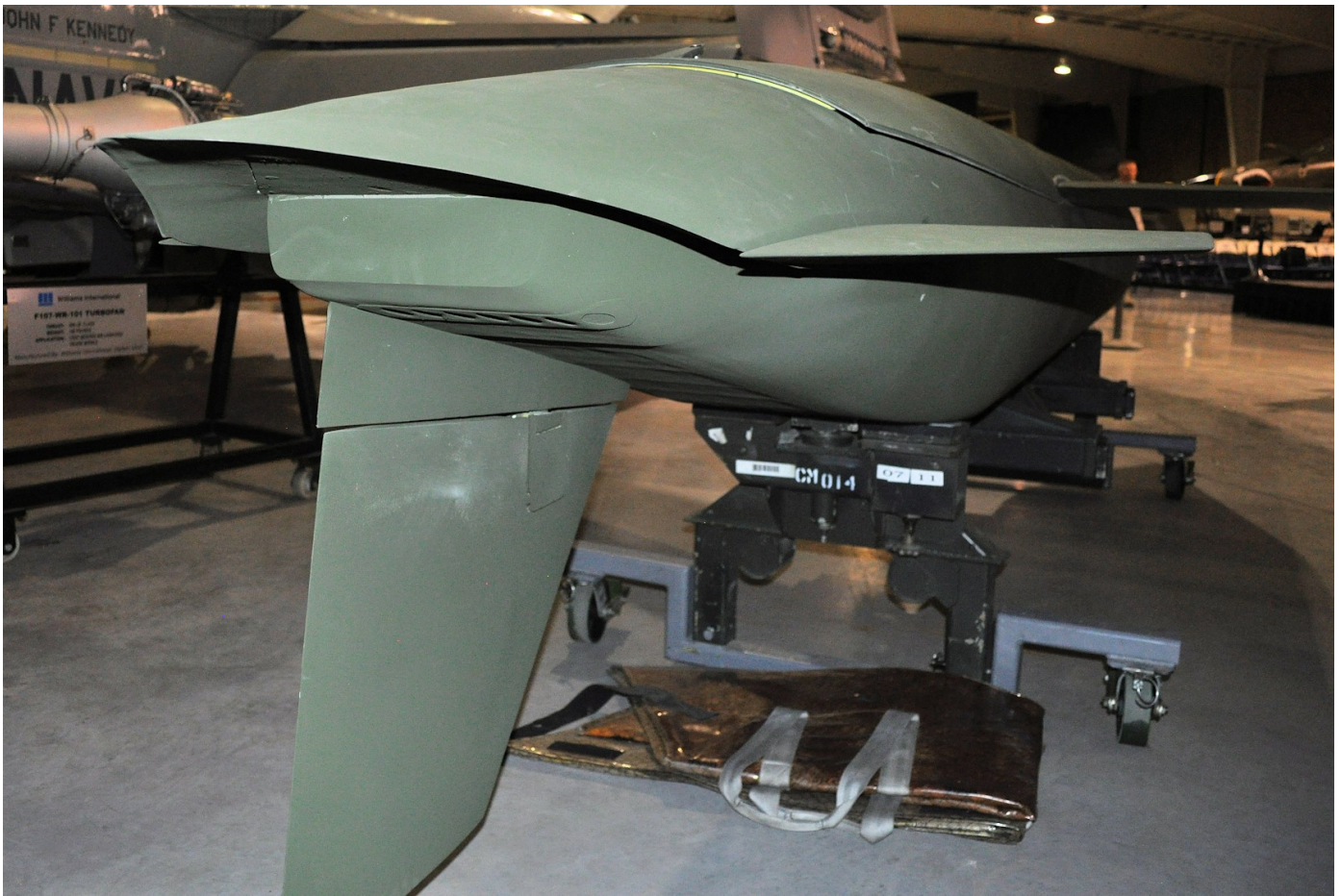
Aft view of the Hill AGM-129. Note that the exhaust nozzle has been closed off. (copyright 2012 Scott Lowther)
