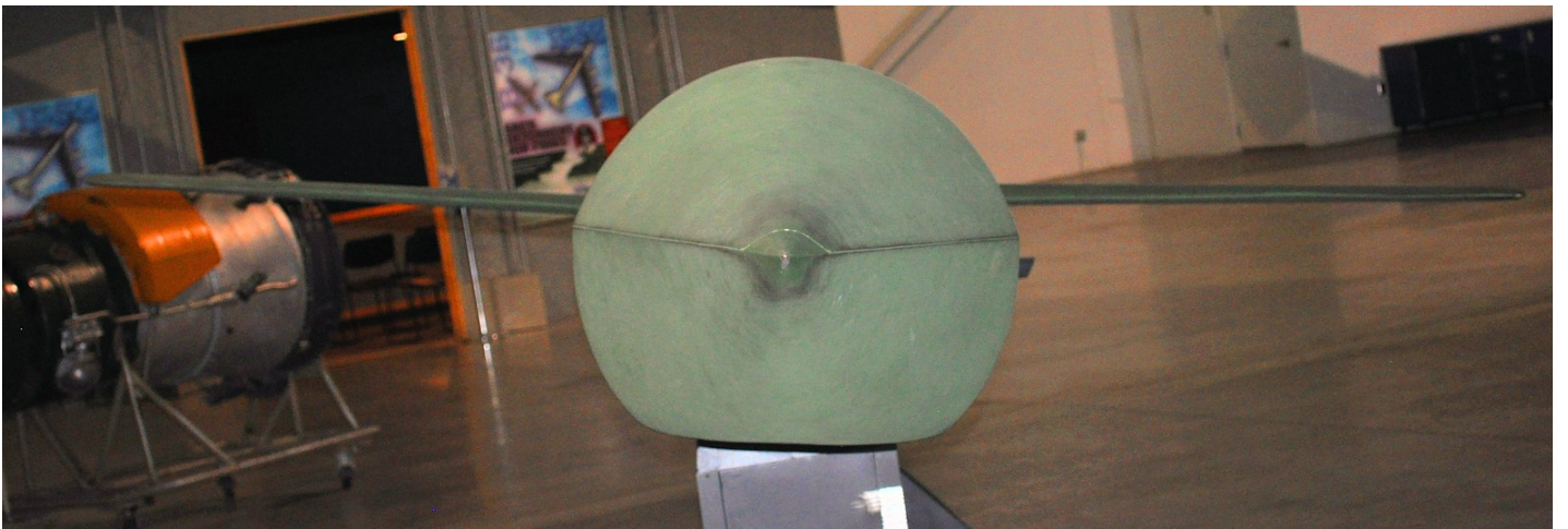
Forward view of the SASM AGM-129A, showing the staggered wing layout to good effect. (copyright 2012 Scott Lowther)
