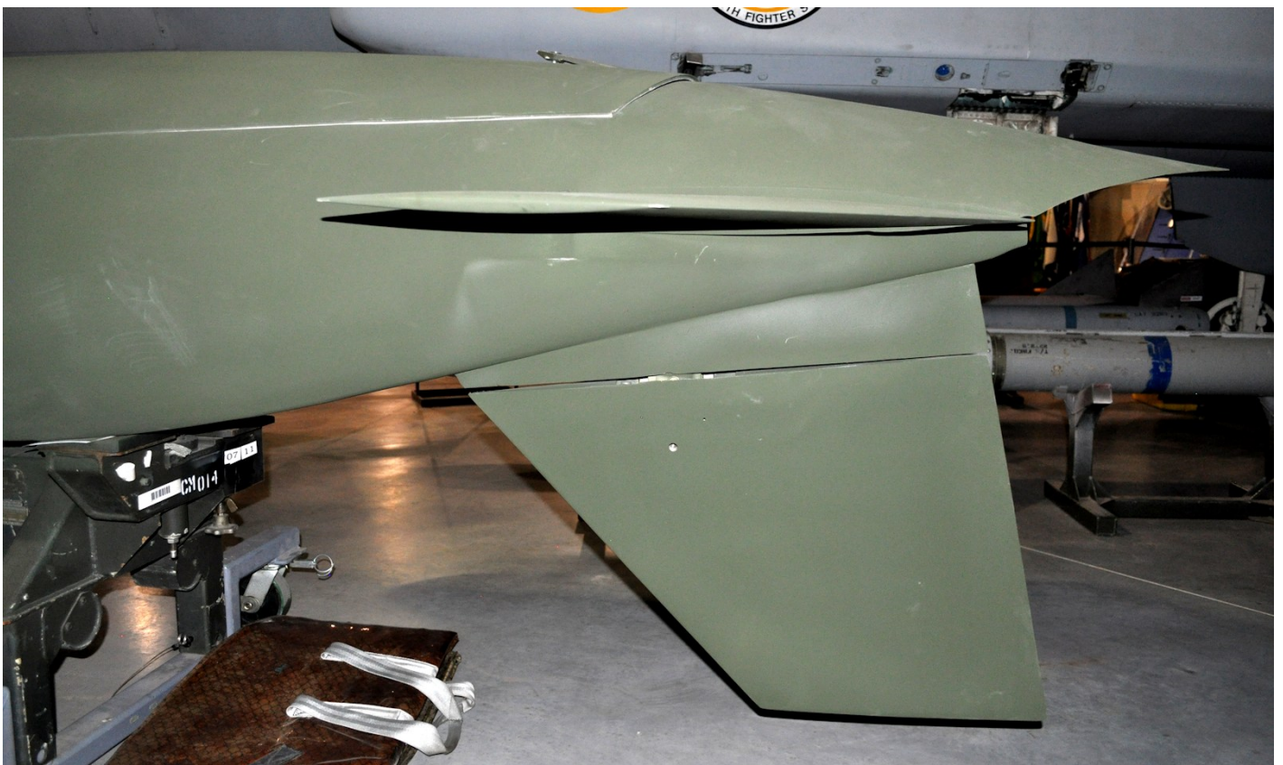
Side view of the tail of the Hill AGM-129. Note that the wing deployment hatch does not seem to be latched down. (copyright 2012 Scott Lowther)
