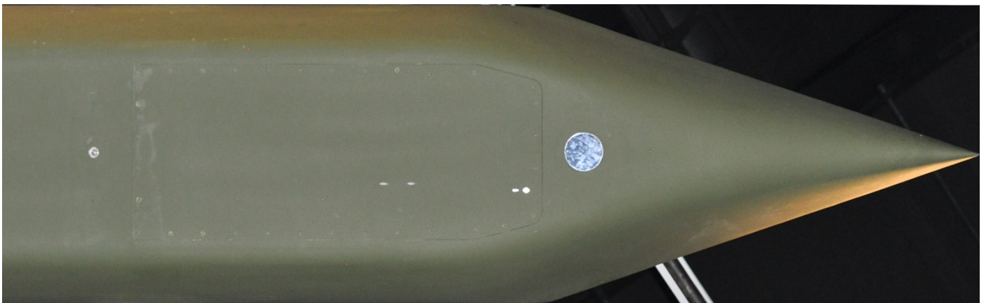
Underside of the nose. Hatch on the underside matched the geometry of the W-80 nuclear device, and is likely how it is installed, accessed and removed from the airframe. Here the circular window for the laser Doppler velocimeter is clearly visible; on other display units it has been painted over. (copyright 2012 Scott Lowther)
